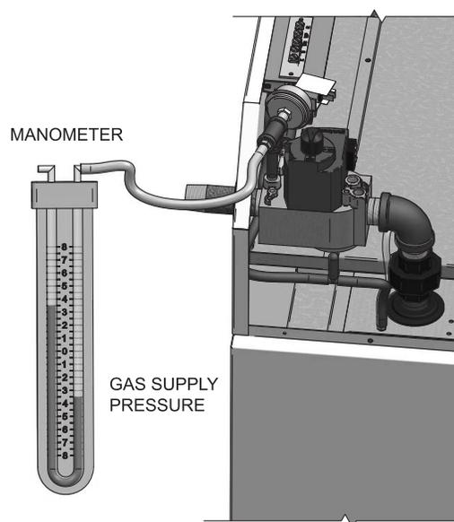
**Figure 3-4** Gas Supply Pressure Measurement - Models ER252 - ER402
